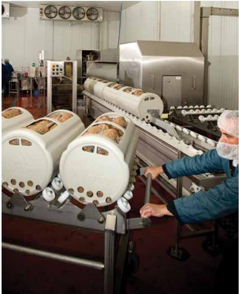
After the cheesesteaks have been packaged, they are loaded into these drums and run through the high-pressure processing equipment. The process is completed in a matter of minutes.
