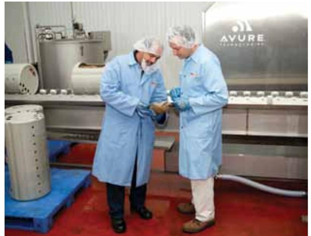
safety, there have been some unanticipated benefits. Astra uses a shrink-wrap, air-tight package for its products. The packages are submerged in water for the HPP process, so employees unloading them from the equipment can easily detect leakers and have the meat repackaged before accidentally being sent to customers.
